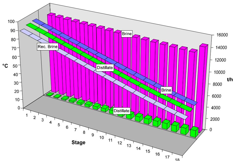
*Fig. 3 Calculation results of the MSF steady-state model for Al Taweelah B power and desalination plant*
