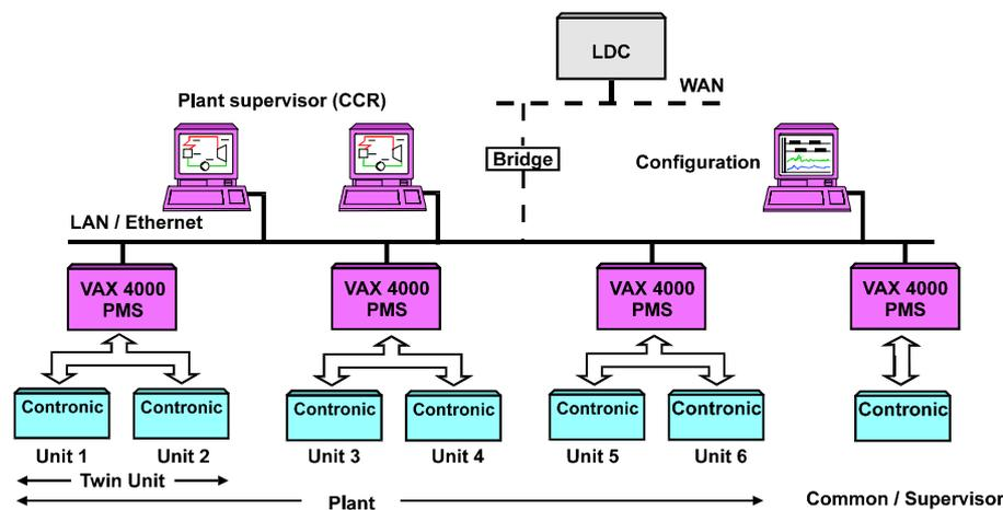
*Fig. 7 Performer Network Configuration of the Al Taweelah B plant*
