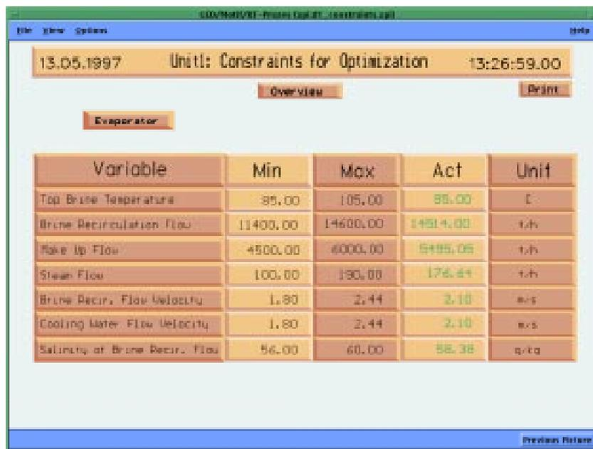
Fig. 9 Faceplate for manually entered constraints
