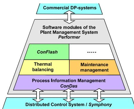
Fig. 6 Modular structure of a plant management system
