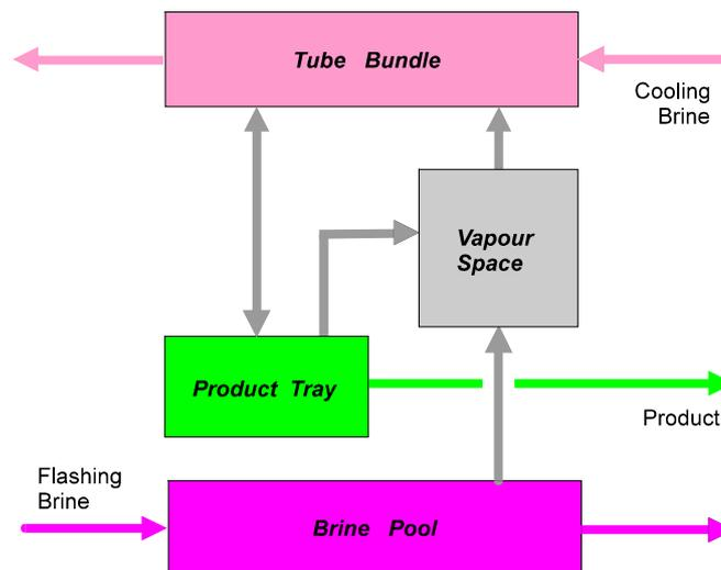
*Fig. 2 Main modules of the stage model*
