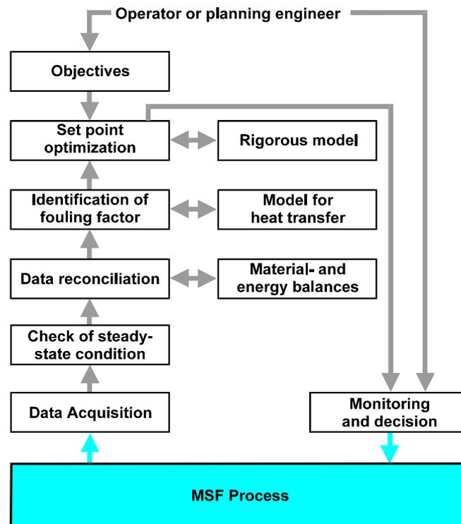
Fig. 4 Signal flow of on-line optimization
