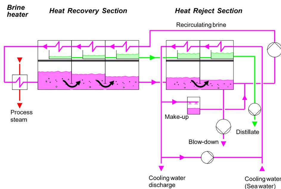
*Fig. 1 Simplified process scheme of a MSF plant*
