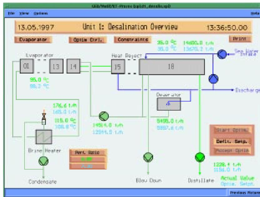
Fig. 10 Display of calculated setpoints
